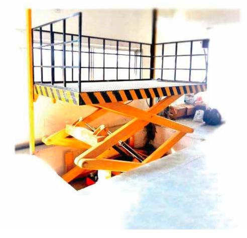
Joist stationary scissor lift is manufactured with higher standard and designed for safe & easy use. Widely used for loading & unloading of the material from one shop floor to another shop floor. It can be installed into the civil pit & other floor as well.
