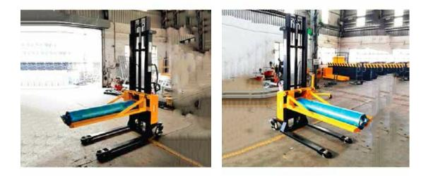
JOIST Reel Stacker is designed for lifting plastic rolls & paper reels, among others. These stackers are suitable for handling anything that rolls & requires to be lifted.
